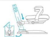
Insert the back steel pipe into the hole on the chair foot, and then install the back steel pipe onto the chair foot with a screw, spring plate and large gasket
