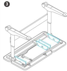
Use 4 screws (M6\*14) to install the drawer bracket on the desktop board assembly.
