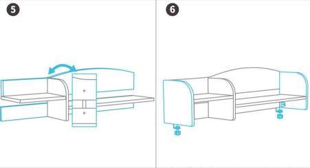
Use M3\*35 screws, screws arbor and lock handles to install the large and small laminates and middle side plates to the upper and lower back plates
